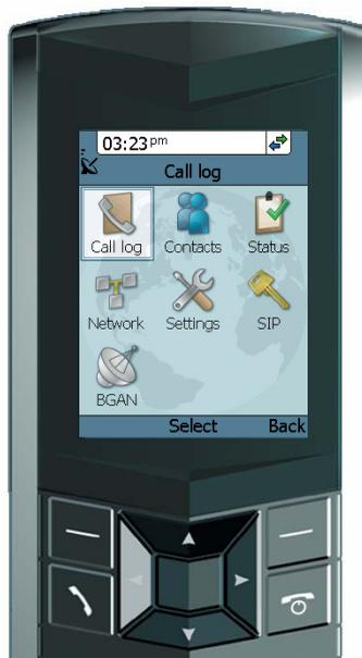
If the handset does not start up, the reason may be that there is no PoE in the LAN interface. If you are connecting to a BGAN terminal, check that the PoE indicator on the terminal lights green for the connected port. For further information, refer to the installation manual for the BGAN terminal.
