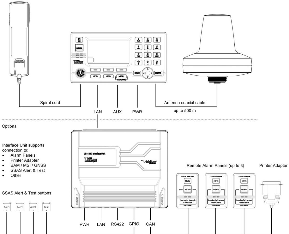
Figure 1: LT-3100S GMDSS system (units and interfaces)
