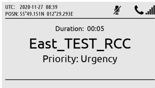
The Safety Call is connected (duration counter will start to count when the RCC has been connected).
