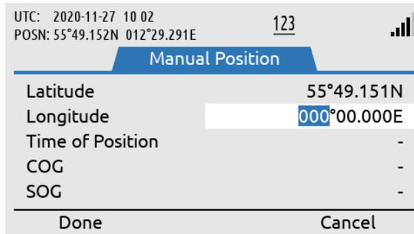
Longitude is configured. Use the soft key 'Done', when Longitude has been entered correctly.
