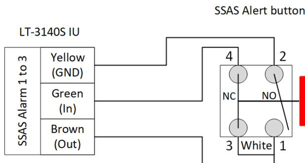
Figure 46: SSAS Alert button wiring diagram
