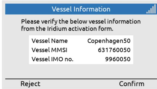
Verify the vessel details, which are provided in the Maritime Safety Service Activation Form (MSSAF) 'Iridium activation form'.
