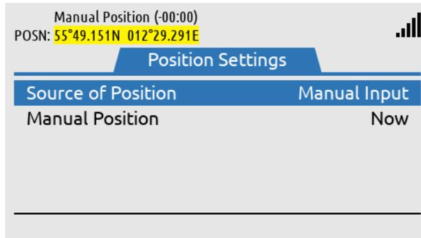
Manual Position is now being used as the position in the system. See information in the status bar (position is colored yellow to indicate low integrity).
