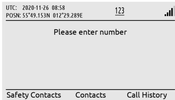
Press the off-hook button (colored green) on the LT-3110S Control Unit. Hereafter press the soft key 'Contacts'.
