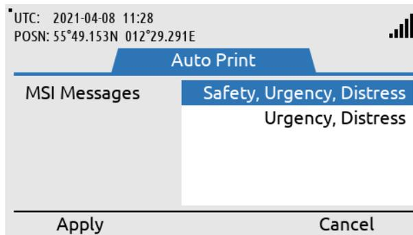
Use the navigation keys and the soft keys to change printing configuration
