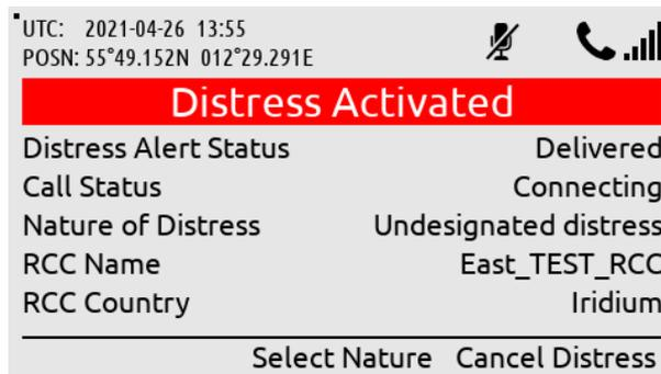
Call Status = Connecting (if Auto-dial = Enabled, then a Distress Call will automatically be established to a RCC).
