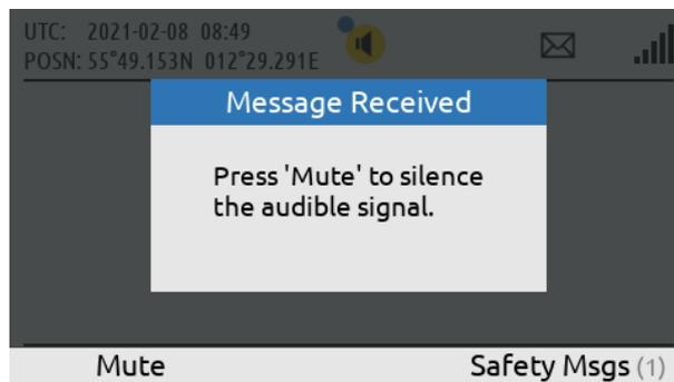
Receiving a Safety Message of Urgency or Distress priority generates an audible alert. Press the soft key 'Mute' to mute the audible alert
