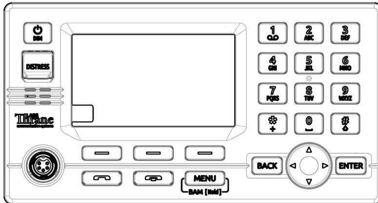
Figure 2: LT-3110S Control Unit (front view)
