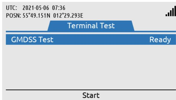
Start the Terminal Test by using the soft key ‘Start’.
