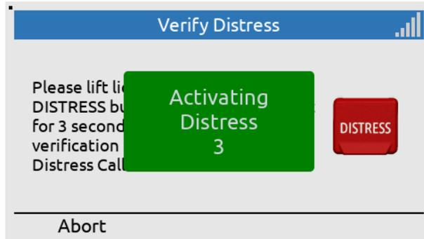
Lift the lid to the DISTRESS button and push the button for a minimum of three seconds (colored green to indicate test).
