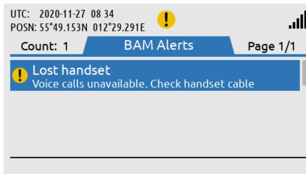
Press the soft key 'ACK Alert' acknowledge the BAM alert.
