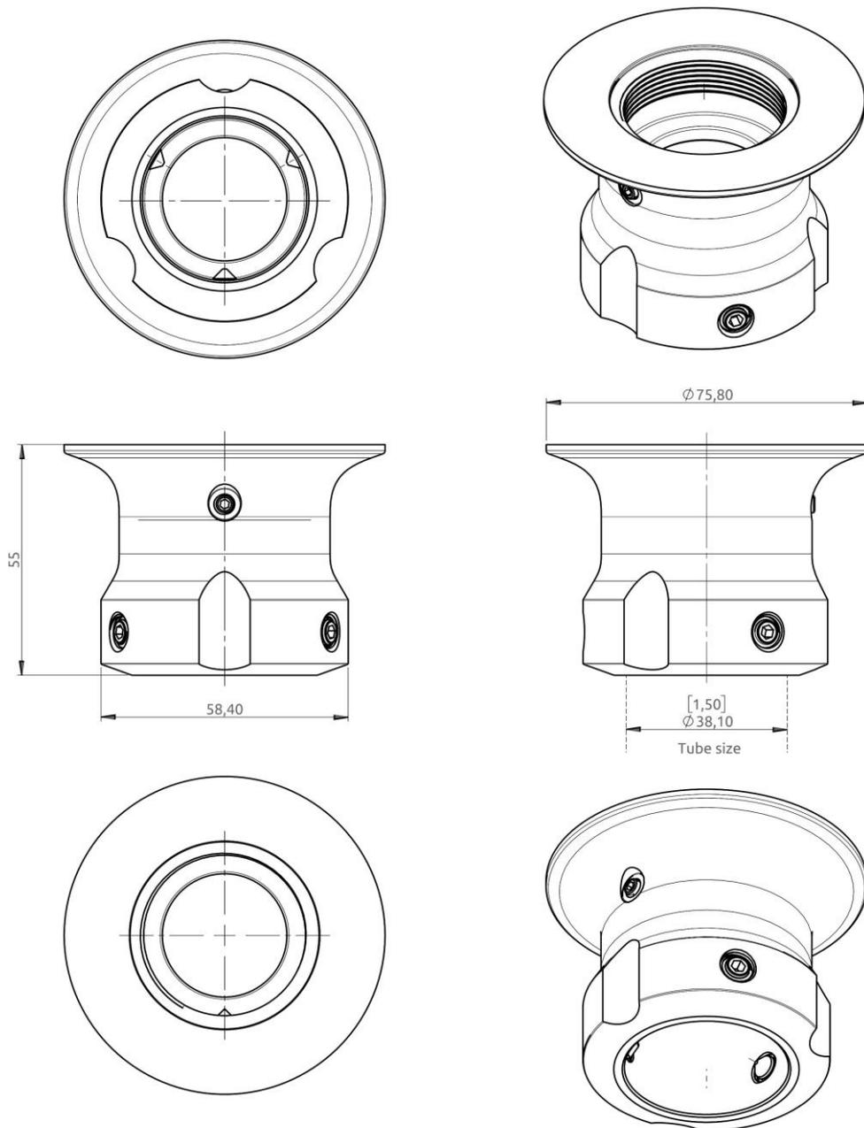
Figure 373: Outline Drawing: Pole Mount (1.5" pipe,  $\varnothing 38.8$  mm), Antenna Unit
