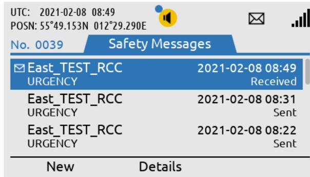
Read the Safety Message by pressing the ENTER button or use the soft key 'Details'.
