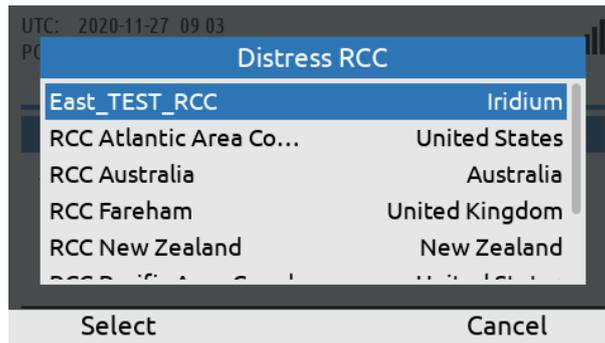
If Distress RCC, Manual has been selected, then the user of the LT-3100S GMDSS system can select an RCC from a list.
