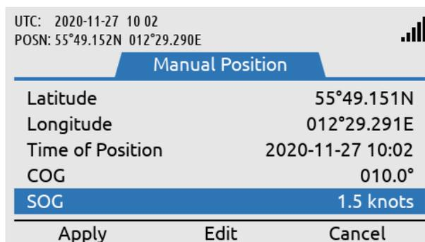
Time of Position, COG, and SOG must be entered. Use soft key 'Apply' when all inputs have been entered correctly.
