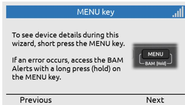
The MENU key can be used to access details (short press) during completion of the Installation Wizard.
