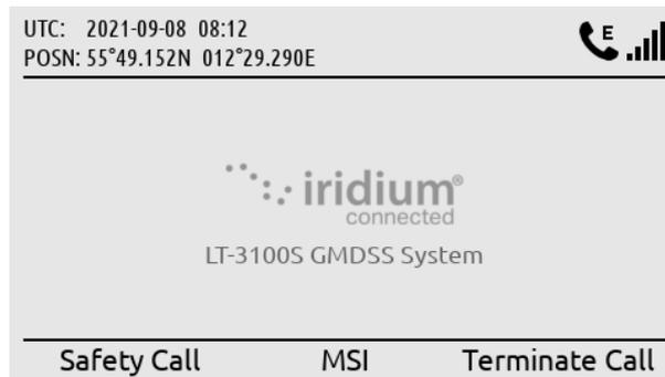
External SIP voice call is using the satellite connection. Can be terminated by using the soft key ‘Terminate Call’.
