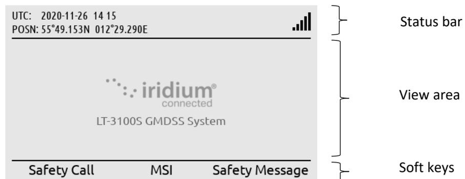
Figure 59: LT-3110S Control Unit (display sections)
