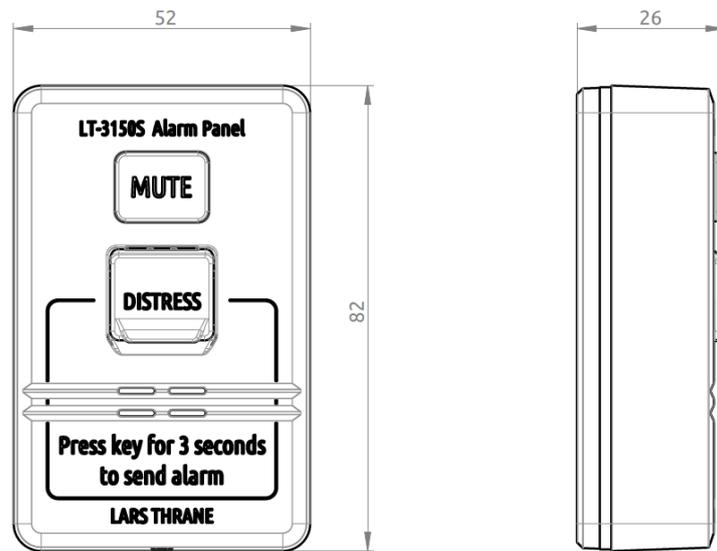
*Figure 371: Outline Drawing: LT-3150S Alarm Panel*
