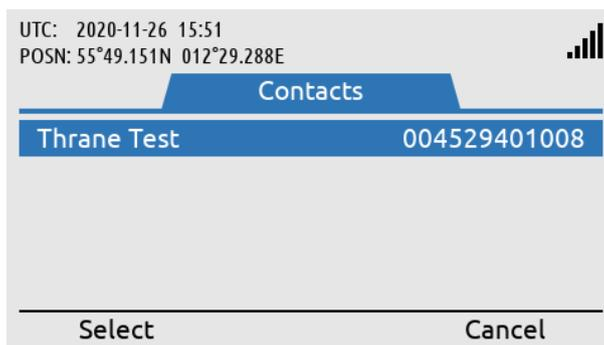
If Contacts has been chosen, then select the contact by using the Navigation key and the soft key 'Select'.
