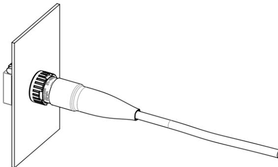
Figure 28: Install SSAS Alert and Test button (3 of 3)
