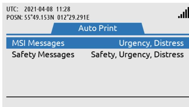
Separate printer configuration of MSI Messages and Safety Messages
