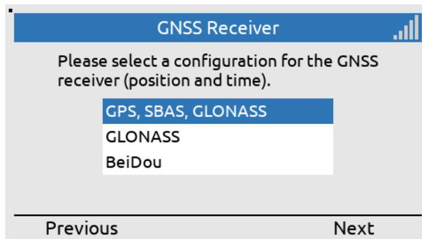
Select GNSS receiver configuration (can be configured via the web server at another time).
