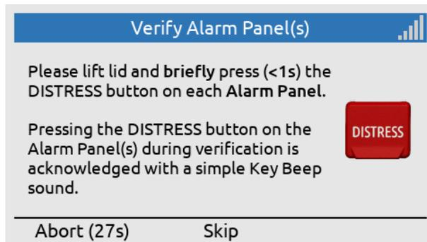
Lift the lid to the DISTRESS button on connected Alarm Panels. Only press the DISTRESS button shortly (< 1 s).
