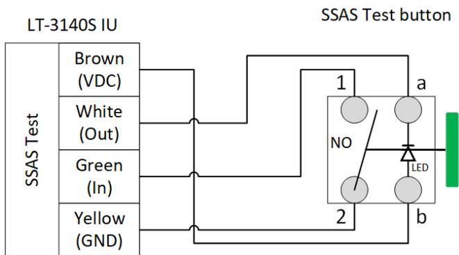
Figure 50: SSAS Test button wiring diagram
