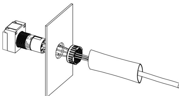
Figure 26: Install SSAS Alert & SSAS Test button (1 of 3)
