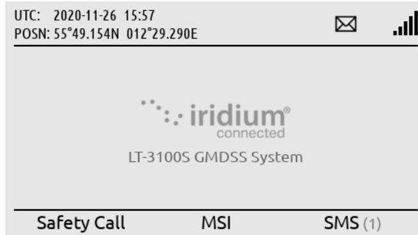
The LT-3100S GMDSS system has received a SMS, see symbol in status bar and soft key 'SMS(1)'.
