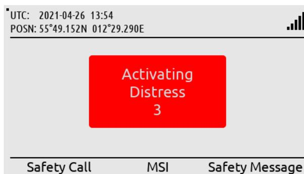
Activation of Distress: DISTRESS button must be held for a minimum of 3 seconds to activate a Distress.
