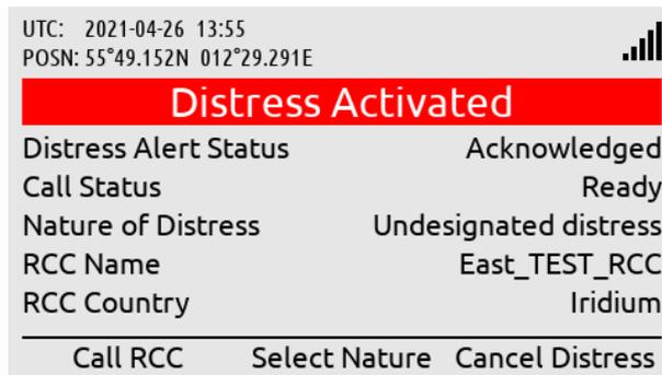
Distress Alert Status = Acknowledged (Distress Alert message has manually been acknowledged by the RCC).
