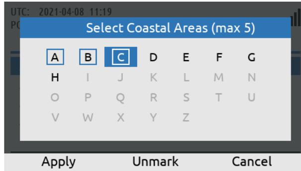
On-going marking of the Coastal Warning Areas to be added. Use the soft key 'Apply' when completed.
