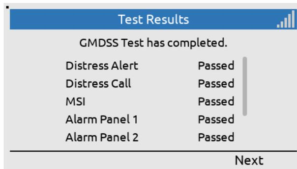
The results of the system verification are listed in the Test Results screen
