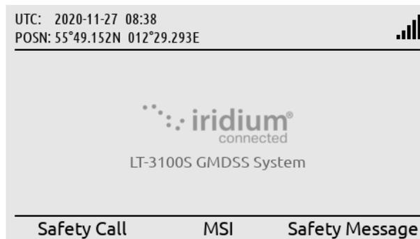
LT-3110S Control Unit, default window. A Safety Call can be initiated by using the soft key 'Safety Call'.
