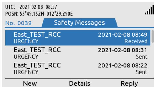
After the Safety Message has been opened (and read) the unread symbol and BAM alert will be removed.
