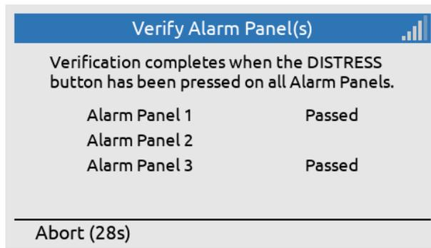
Press the DISTRESS button on all connected Alarm Panels with a short press (< 1 s).
