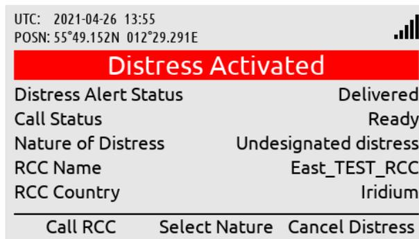
Call Status = Ready (Distress Call has been disconnected to the RCC). Use soft key 'Call RCC' to activate a new Distress Call.
