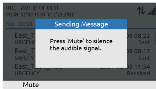
Sending a Safety Message of Urgency priority generates an audible alert. Press the soft key 'Mute' to mute the audible alert
