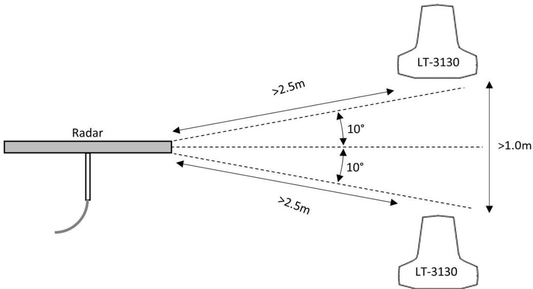
Figure 13: LT-3130 Antenna Unit (avoid the radar beam)
