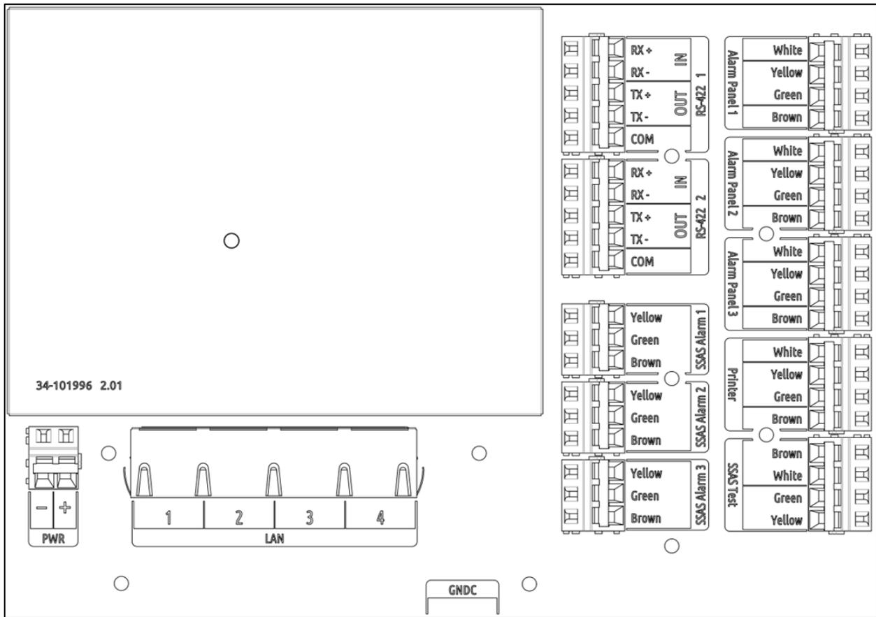
Figure 42: LT-3140S Interface Unit (with interface labels)
