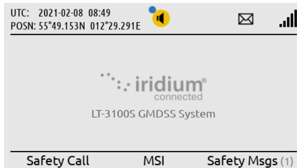
Upon muting, the LT-3110S Control Unit returns to the default window. The Safety Message can be read by using the soft key 'Safety Msgs (1)'.
