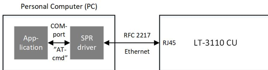
Figure 254: LT-3100S GMDSS system is supporting RFC 2217 (Serial over Ethernet)
