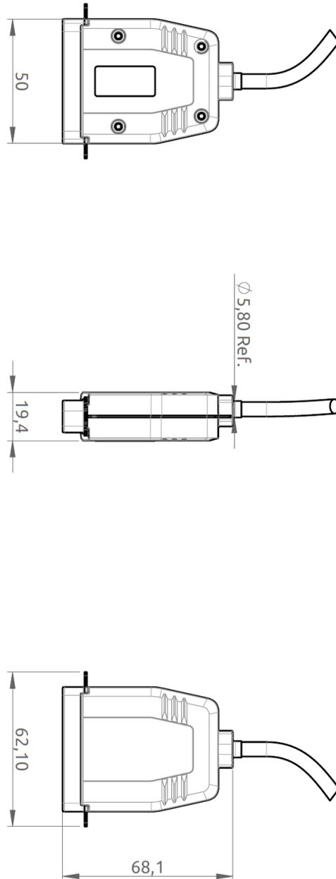
*Figure 372: Outline Drawing: LT-3160S Printer Adapter*
