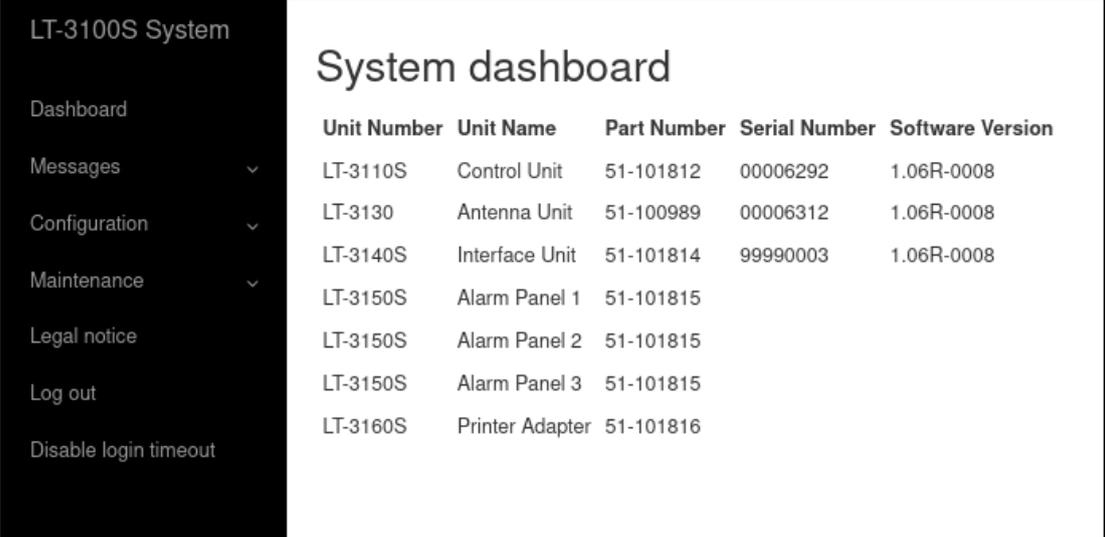
The screenshot shows the 'System dashboard' for the LT-3100S System. On the left is a dark sidebar with navigation links: Dashboard, Messages (with a dropdown arrow), Configuration (with a dropdown arrow), Maintenance (with a dropdown arrow), Legal notice, Log out, and Disable login timeout. The main content area is titled 'System dashboard' and contains a table with the following data:
