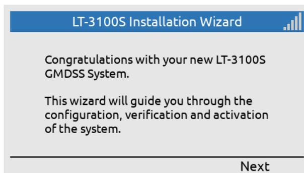
The Installation Wizard will be displayed when powering up the system initially, and until activation completed.
