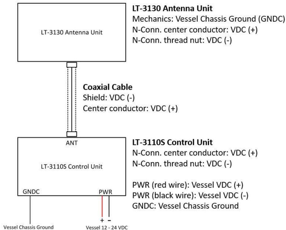
Figure 54: Definitions of VDC (+), VDC (-), and GNDC
