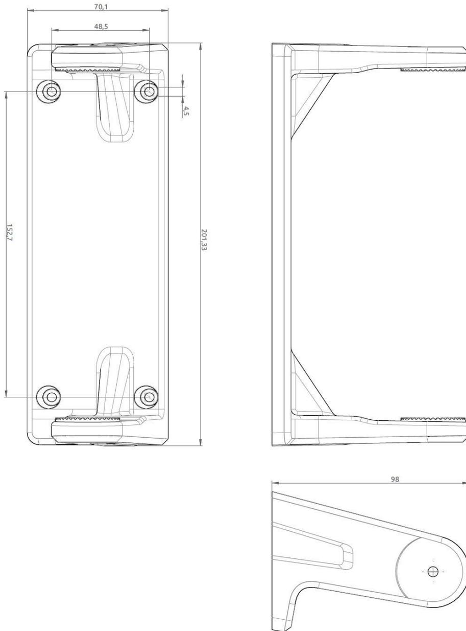
*Figure 367: Outline Drawing: Bracket Mount, Control Unit*
