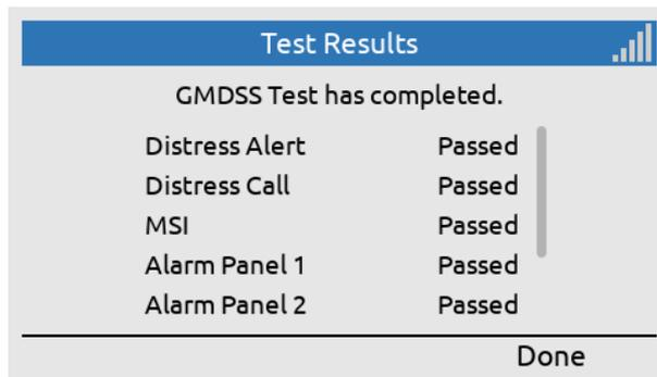
Upon finalizing the Terminal Test, the Test Results will be displayed.
