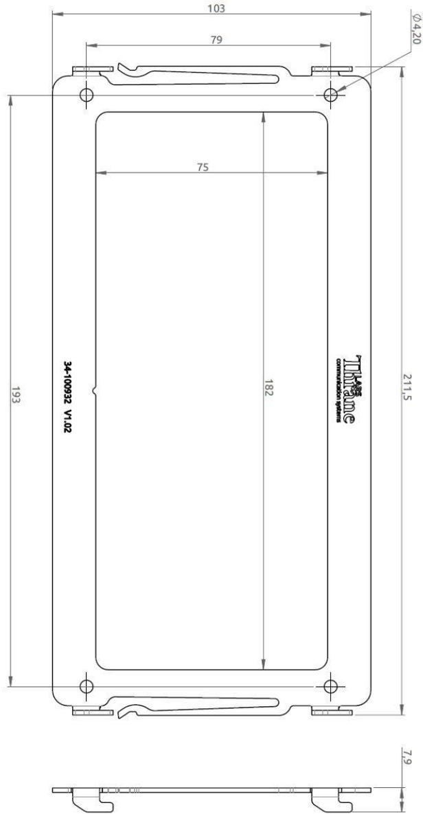
Figure 368: Outline Drawing: Flush Mount, Control Unit
