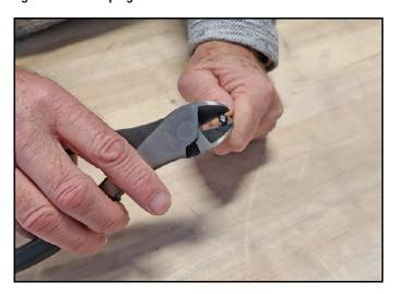
3. Place the metal ferrule onto the cable.
