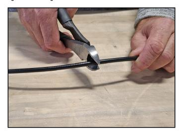
2. Since cutting the cable can deform the end, gently round the end of the cable. Also make sure the center conductor is centered within the cable.
