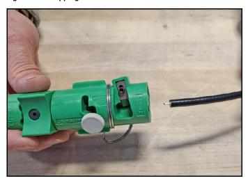
Figure 51: Cable Stripped, Exposing Dielectric
