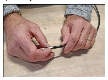
4. Insert the end of the cable into the #1 end of the CST-240 stripping tool. Depress the cutting blade using your thumb, then rotate the tool clockwise around the cable until the tool turns easily. The end of the cable should now be stripped to expose the center conductor.
