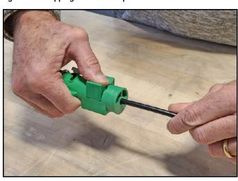
**Note:** Carefully remove any residual plastic from the center conductor, if necessary.
