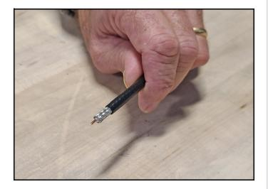
6. Using the DBT-U deburr tool, deburr and chamfer the center conductor. Avoid nicking the aluminum tape covering the dielectric.
